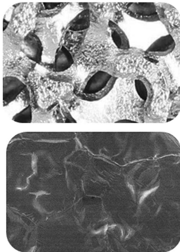
**Figure 1.** The deeply porous titanium scaffold (upper figure  $\times 30$  magnification; lower figure  $\times 1000$  magnification; figures courtesy of Nanovis, with permission).
