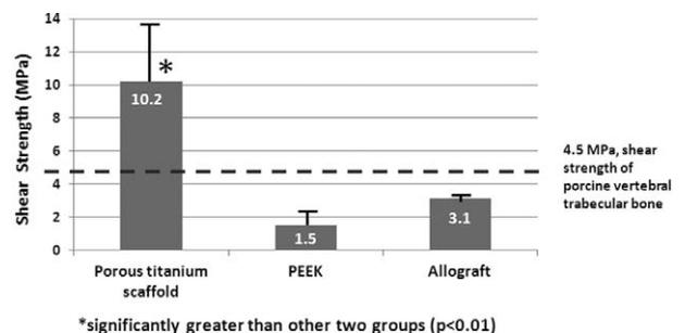
**Figure 4.** Mean pin push-out strength was significantly greater in the porous titanium group ( $P < 0.05$ ) than in either of the other two groups. The shear strength of porous titanium group is also significantly higher than that of mature porcine trabecular bone ( $P < 0.05$ ). Values are means and the bars represent the standard deviations. PEEK indicates polyetheretherketone.
