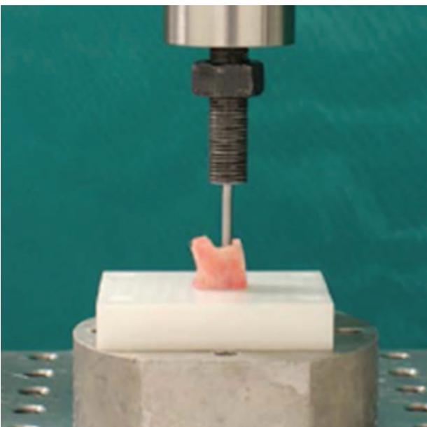
**Figure 3.** Mechanical push-out testing was performed on all samples to determine the shear strength of the implant-bone interface.
