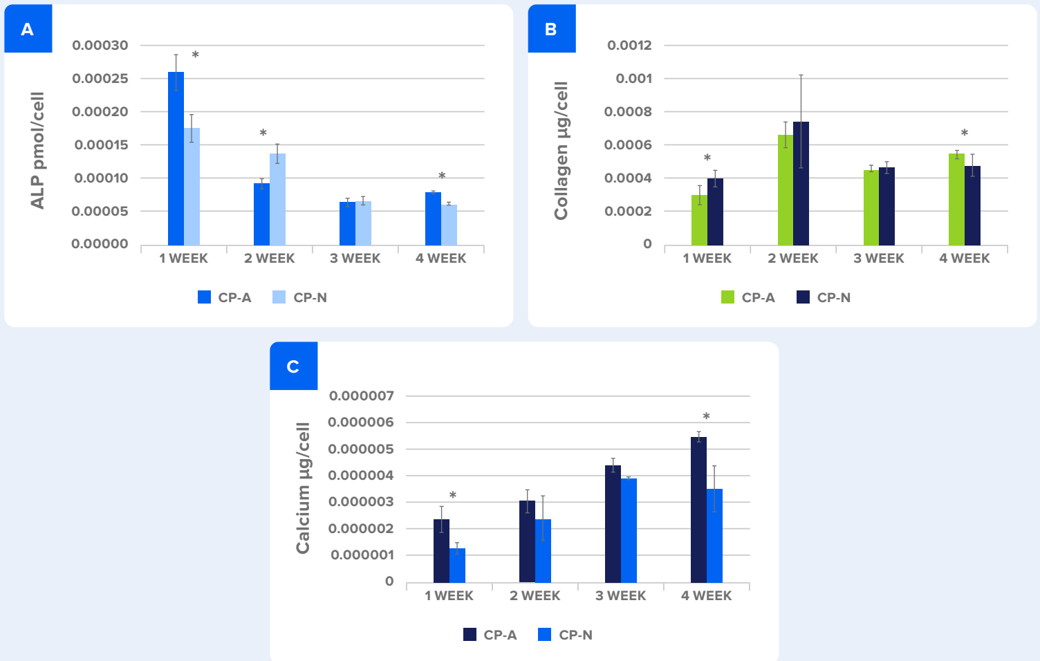
Figure 1 - A) Alkaline phosphatase activity, B) Intracellular collagen production, C) Calcium deposition from human osteoblast cultures at 1, 2, 3, and 4 weeks of culture. All results are presented on a per cell basis. CP-A = anodized nanotubes CP Ti; CP-N control surface non-treated CP Ti. The asterisk mark (*) Indicates significant differences based on a Student's T-test, p-value<0.05.
